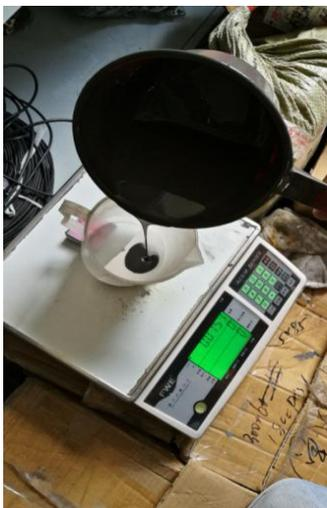
7. 2<sup>nd</sup> Stirring: Please stir evenly. (The silicone turns into gray after 10 minutes' stirring.) Make sure the tool is clean before stirring.
