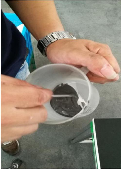
8. 2nd potting: Pour 30g(1.06 oz) on electric board. Evenly pour silicone on electric board and make sure all electronic components totally glued. **Attentions not get silicone into terminals.** Keep the electric board flat, wait till silicone dried (become gel).
