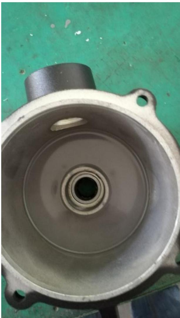
Clean the residue in container, as it will also dry, can't be used for 2<sup>nd</sup> potting.
